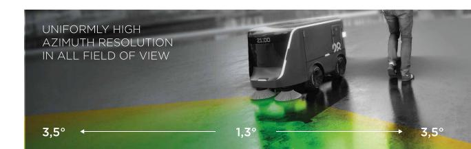
Obstacles detection in any lighting and weather conditions
